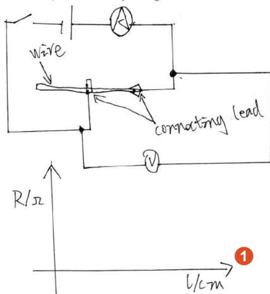
1 The candidate draws a workable circuit diagram including the correct circuit symbols.
