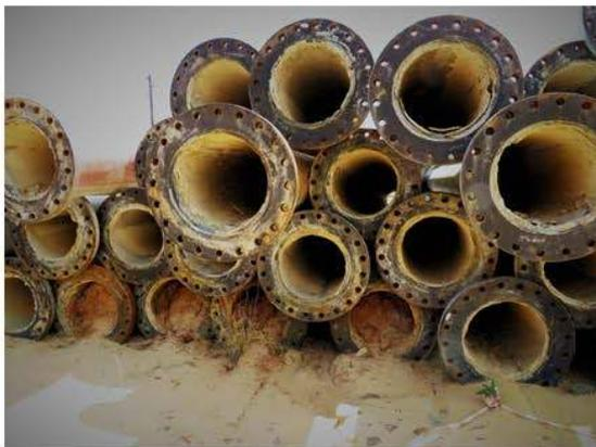
Pipes that carry the harmful water from the mines and tailings to the dam sites litter the landscape. As the photographs show they have filled with layers of heavy metals and other deposits.
