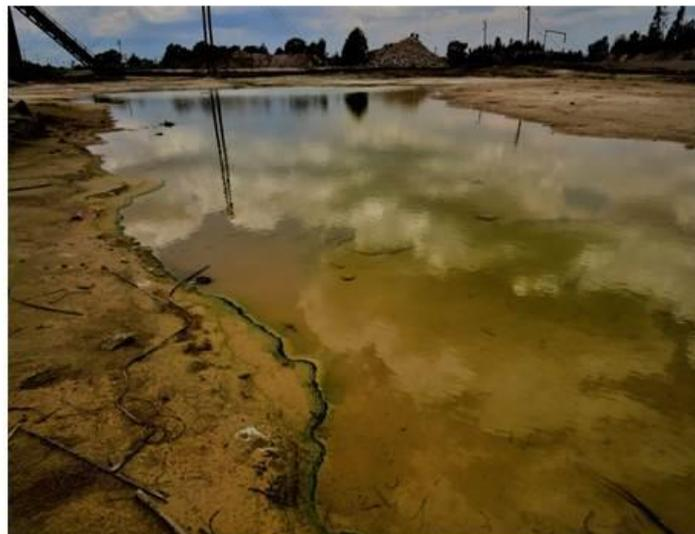
The high level of copper in the water can be seen as a green residue around the edges of this puddle in a tailing.
